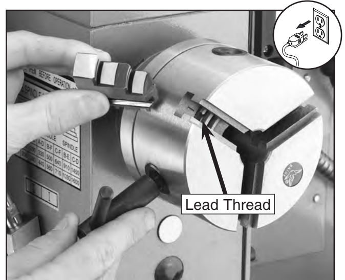
Figure 14. Arrow points to the lead of the scroll.
